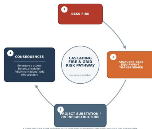
Figure 7.1: Potential escalation from a BESS fire into adjacent equipment, project HV infrastructure and wider operational consequences.
